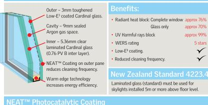
Silicone Dioxide/Titanium Dioxide coating reacts with the sun's UV rays to decompose surface organic dirt before rinsing away with the next shower of rain, thereby reducing cleaning frequency.
